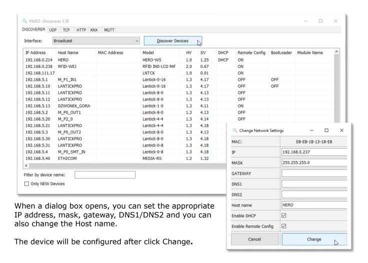
If Remote Config is disabled (enabled by default), it is necessary to configure the device by changing the subnet of the computer (section 6.2).
