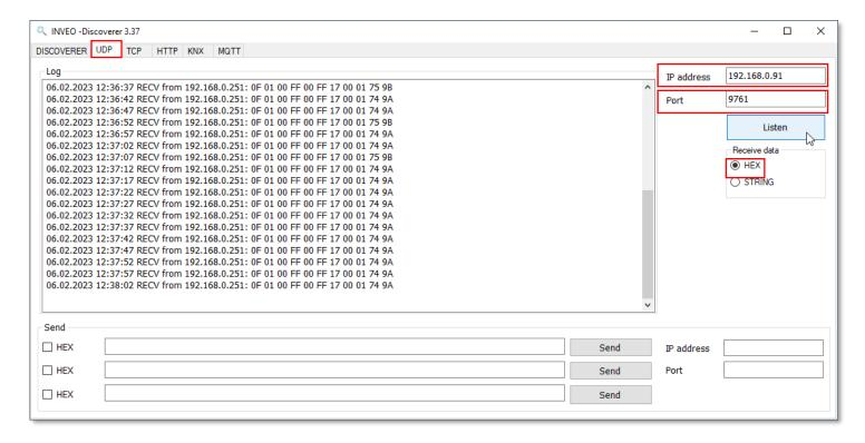
To test the following message types: Status, Mac+status you should select Status or Mac+status respectively in the Channel tab. The next step is to start Inveo Discoverer and go to the TCP tab. In the IP address and Port windows, enter the same values as in the Network tab. In the Receive Data window, select the STRING option. Finally, click on the Listen button.
