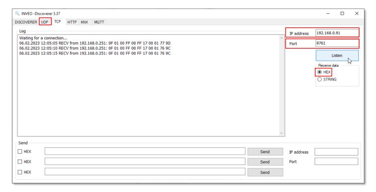
When testing UDP messages, select UDP Ch:x in the Channel tab. Then switch to the UDP tab in Inveo Discoverer. In the IP address and Port boxes, enter the same values as the Network tab. In the Receive Data box, select the HEX option. Finally, click on the Listen button.
