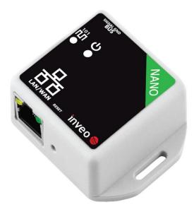
The module is equipped with LEDs that indicate the power supply of the module and the moment of temperature reading from the sensor.
