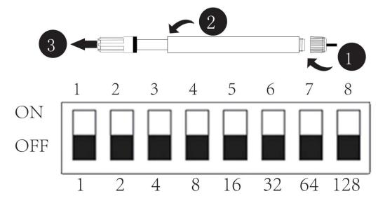
Calculation: the DIP digits1~8 respectively correspond to number 1, 2, 4, 8, 16, 32, 64, 128(as shown in the figure above); Add all the values corresponding to the DIP digits 1-8 dialed to NO, that is the value of the address code. For example:
