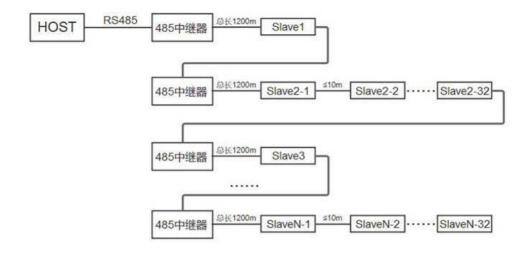
3) parallel: up to 16485 repeaters are supported and connected to the same 485 input device, and up to 128 devices are supported.
