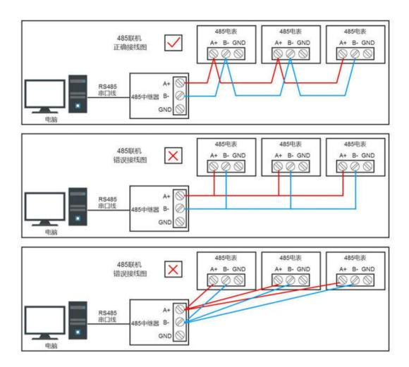
1) single repeater: point-to-point connection of a 485 output device extends the communication distance by 1200m; point-to-multipoint connection of 32485 output devices with adjacent 485 devices not exceeding 10m extends the total bus length by 1200m.
