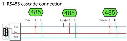
The COM port of a computer is generally RS232, so you need a 232-485 converter for connection(an active and isolated converter is recommended for industrial environments). After conversion, RS485 has A and B two wires, A is connected to the board A terminal, and B is connected to the board B terminal, the 485 shield can be connected to GND. If there are more equipment, it is recommended to use shielded twisted-pair cable and a chain network structure.
