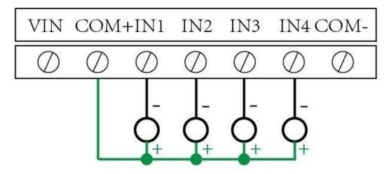
3.2. Wiring diagram of passive switch (dry contact)
