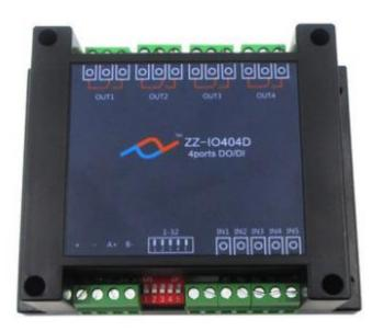
The module adopts the standard Modbus RTU protocol, the communication interface supports RS485 or RS232, and supports communication baud rates of 2400, 4800, 9600, 19200, 38400 (default 9600). Each relay output is independent and can be connected to different load devices, such as 220V electric lights, 24V solenoid valves, etc. Both AC and DC devices can be controlled. Each relay output contact is isolated, and can set 0-255 device addresses. It also supports flash on/off function.
